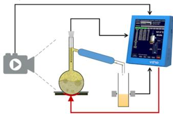
The entire test procedure is fully automated: position of the flask, its heating, condenser and receiver temperatures regulation, measuring vapor temperatures and volume, detecting IBP and FBP, rate control, perform barometric correction and recording all data. At test completion, the heater is automatically lowered and cooled down quickly. Results are displayed, sayed, printed, sent to LIMS or USB.
